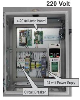
View of the variable rate controller, with Emerson variable frequency control
